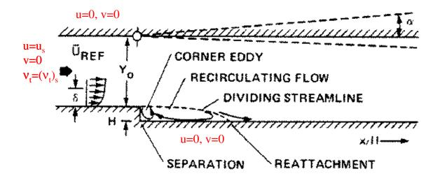
TUNNEL GEOMETRY: H = 1.27 cm, y<sub>0</sub> = 8H
