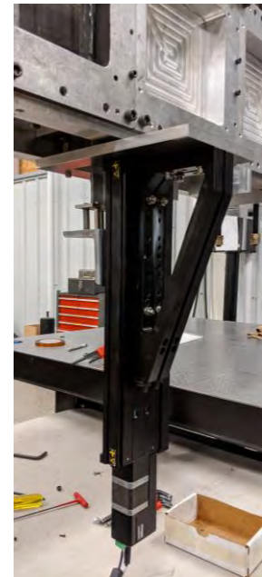
Figure 18. Zaber stage traverse system
