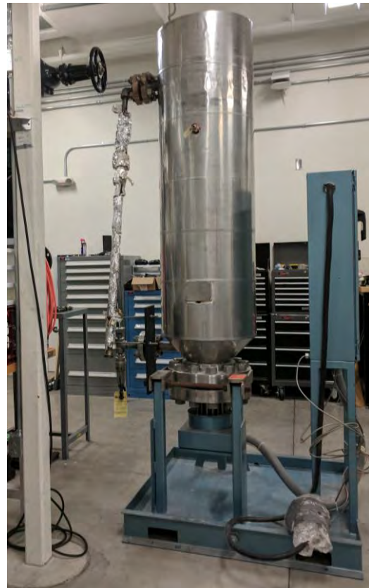
Figure 7. Electric air heater in GDL
