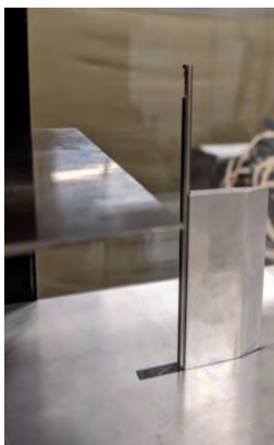
Figure 20. TAT probe mounted in tunnel
