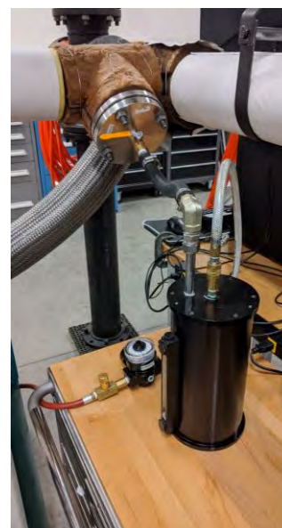
Figure 37. Secondary seeding configuration with Laskin Nozzle seeder
