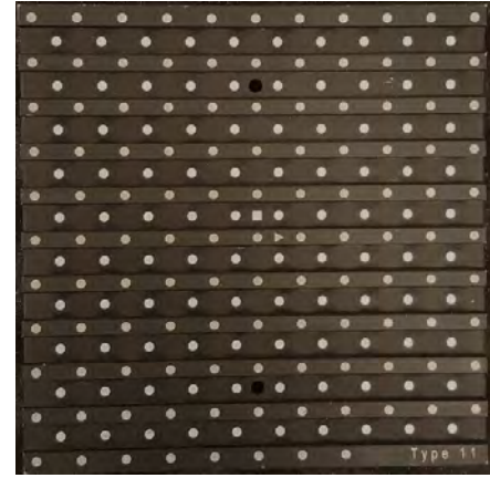
Figure 23. LaVision two-level calibration plate (Type 11).
