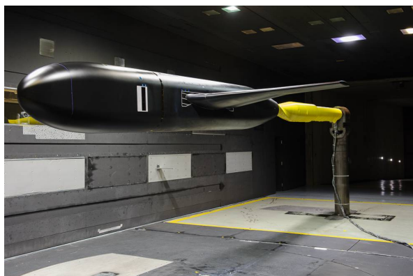
Figure 1. Port-side image of the wing-fuselage junction model installed in the 14- by 22-Foot Subsonic Tunnel.
