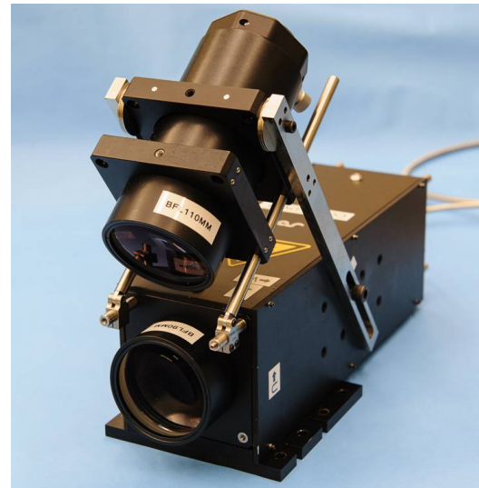
Figure 8. Photograph of the LDV probe head with off-axis receiving optics.
