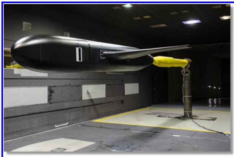
Fig. 1 8% Junction Flow Model installed in the 14- by 22-Foot Subsonic Wind Tunnel.
