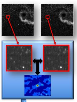
Particles in the flow are exposed by two laser pulses separated in time and imaged using CCD or CMOS cameras.
