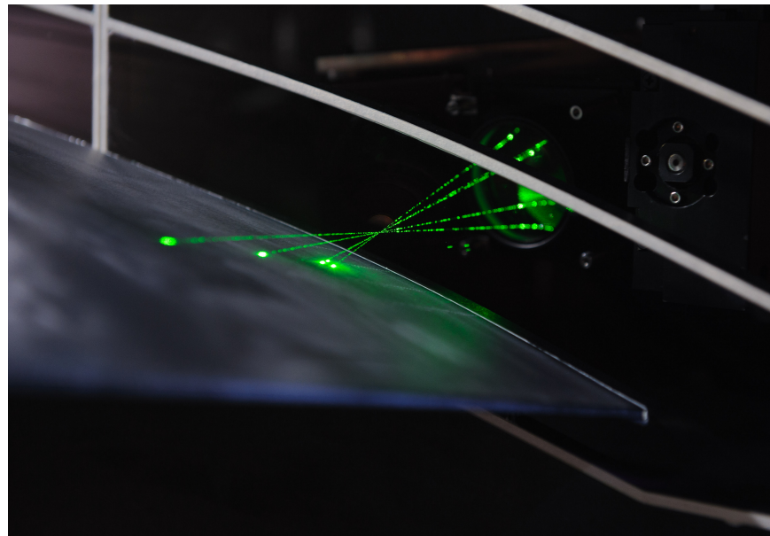
LDV system installed at the wing trailing edge
