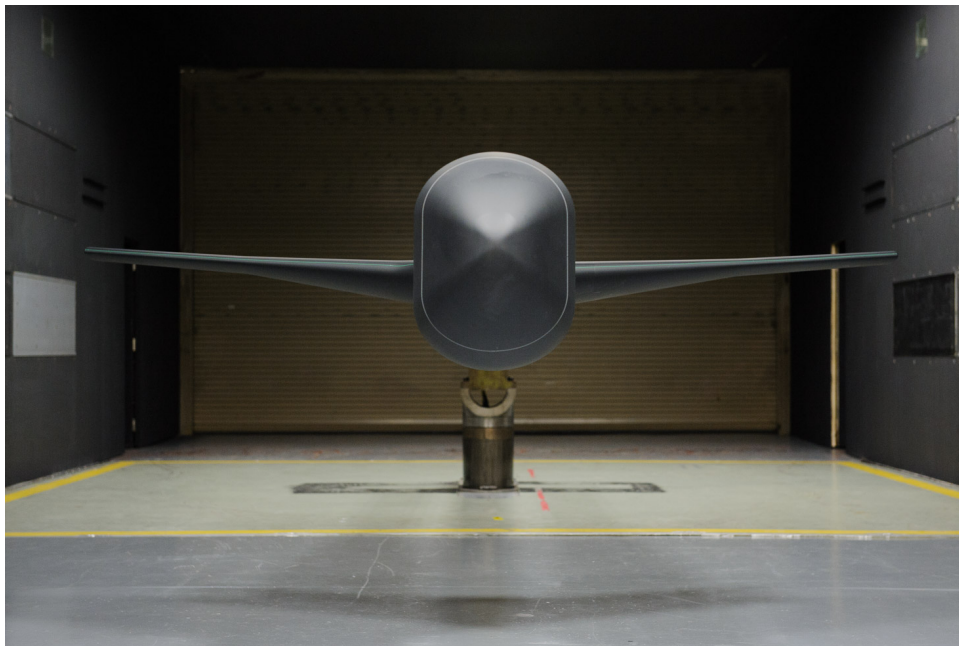
Figure 2. Front-view image of the Juncture-Flow Model installed in the 14x22 Subsonic Wind Tunnel.
