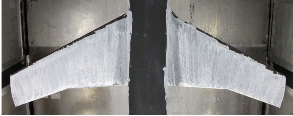
(a) Oil-flow visualization in the Virginia Tech Stability Tunnel at Re_c = 0.62 million.
