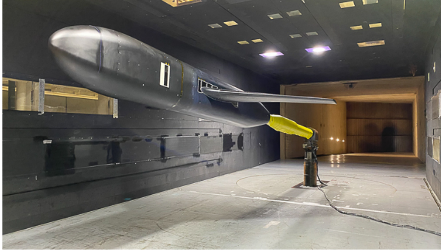
Figure 2: Port-side view of the wing-fuselage junction model installed in the 14- by 22-Foot Subsonic Tunnel.
