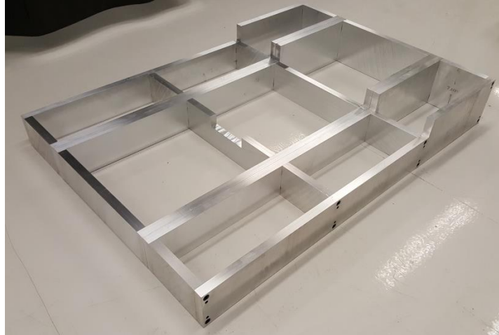
Figure 9 Supporting structure for ramp model that provides the necessary 0.152 m (6 in) of vertical offset required for optical access to the recovery region.
