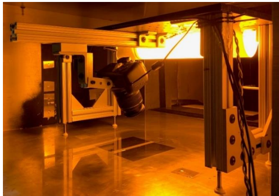
Figure 1 Photograph of test fixture, shown in place at the X = -0.678 m location, developed to illuminate and photograph the interferogram images.
