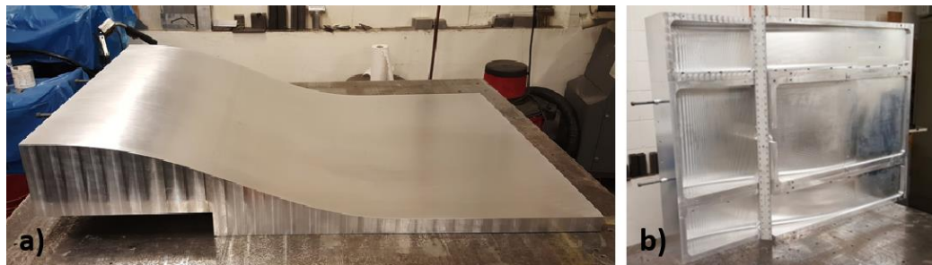
Figure A.2 Photographs of the top (a) and bottom (b) assembled ramp model just after polishing showing the three separate sections bolted together
