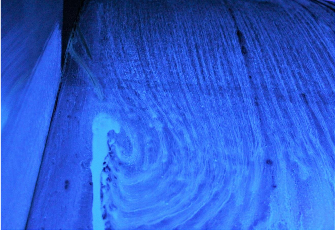
Figure 27 Surface flow visualization for Case C with incoming flow from top to bottom (Test 1, July 2019)
